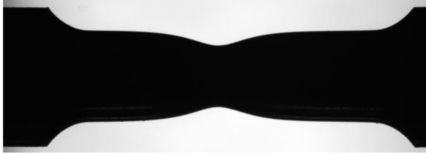
Figure 1.9: A silhouette photo of an initially cylindrical specimen from steel bar that has necked during QS loading.
