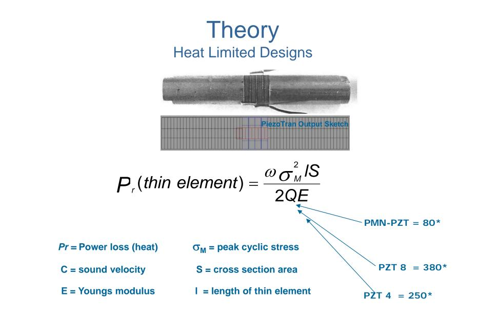
Q : Defined as the ratio of the energy stored to that lost per cycle multiplied by 2  $\pi$
