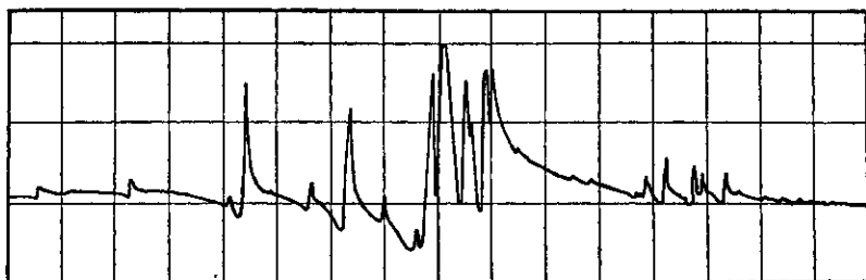
FIG. 85.—Resonance curve for an X -cut 1,500 kc/sec quartz plate in thickness vibration, from Bechmann, 37 showing many resonant frequencies over a range of about 30 kc/sec.
