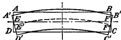
FIG. 16.—A rectangular plate ABCD bent by flexure into the form A'B'C'D' . The plane of the figure is the plane of flexure. The surface through EF normal to the plane of the figure is the neutral surface.
