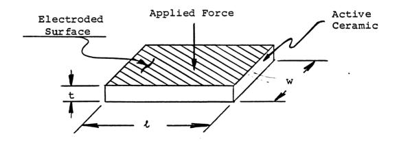
The energy of a charged dielectric plate is given by equation (1):
