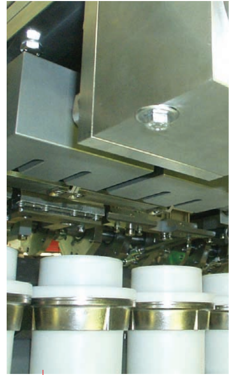
Ultrasonic welding for high-speed tube filling line.
