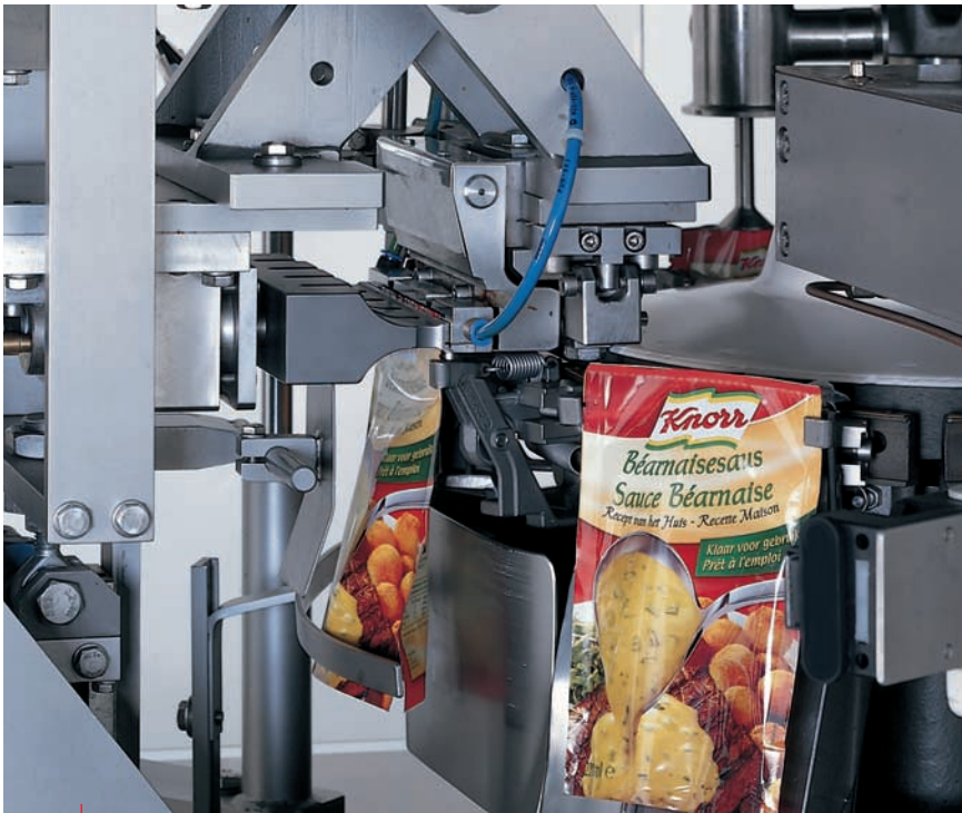
Ultrasonic sealing through top seal product contamination in an SUP production line.
