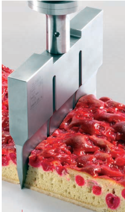
Ultrasonic technology utilized for food cutting applications.
