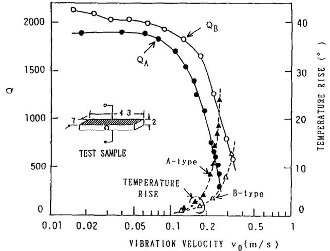
Fig. 2. Vibrational velocity dependence of the quality factor and temperature rise for both resonance and antiresonance of a PZT ceramic longitudinally vibrating transducer.
