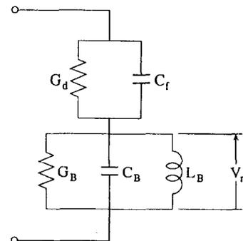
Fig. 1. Advanced impedance-type equivalent electric circuit.
