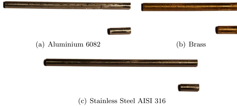
Figure 4.27: Rod horns used in the half and full wavelength assemblies
