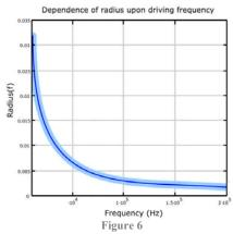
Variation in cavitation bubble radius as a function of driving frequency.
