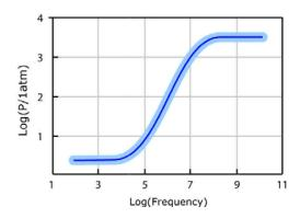
$Figure \ 5$  The threshold of cavitation of filtered tap water is strongly a function of frequency, especially above 100kHz.  $^{6.7.8}$
