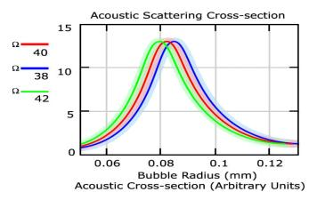
Figure 3 The acoustic interaction cross-section as a function of bubble radius (mm) for 40kHz ultrasonics.  $\Omega_{40}$  is the cross-section at 40kHz,  $\Omega_{38}$  is the cross section at 38kHz, and  $\Omega_{42}$  at 42kHz. This demonstrates how sweeping the ultrasonic frequency creates a band over which a bubble population is excited.
