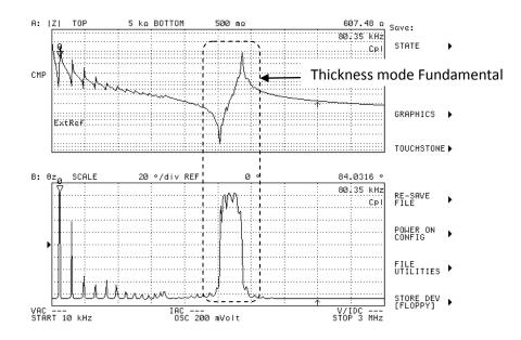
*Figure 5: Fundamental Thickness Mode Resonance*. The thickness mode resonance is much wider and stronger than the radial mode harmonics.
