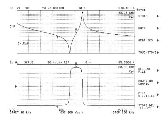
**Figure 3:** Fundamental Radial Resonance. The fundamental resonance consists of a resonant and antiresonant frequency. The impedance (top curve) drops to a minimum at the resonant frequency and rises to a maximum at the antiresonant frequency. The phase angle (bottom curve) rises to a maximum value roughly at the center of the resonance.
