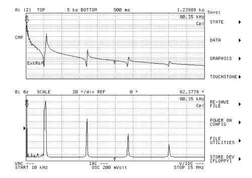
*Figure 7: Thickness Mode Harmonics.* The  $3^{rd}$ ,  $5^{th}$ , and  $7^{th}$  harmonics are progressively weaker than the fundamental thickness mode.
