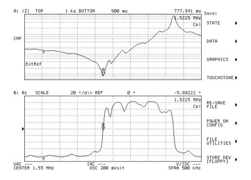
**Figure 6:** Fundamental Thickness Mode and Nearby Radial Mode Harmonics. Note the spacing of the "serrations" in the impedance (upper curve) and phase angle (lower curve) in the radial mode matches that of the radial mode harmonics seen to the left (lower frequency).
