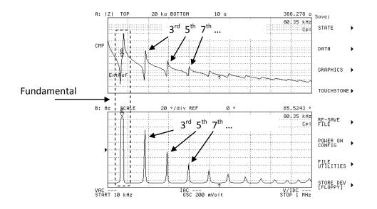
*Figure 4: Radial Frequency Harmonics.* The fundamental resonance is followed by a series of odd harmonics at progressively higher frequencies. The strength of the harmonic and the spacing between the resonances decreases as the order increases.
