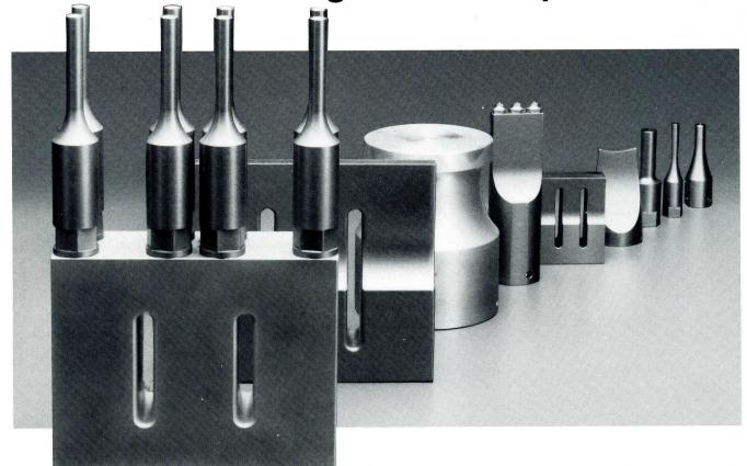
Ultrasonic welding horns and tips are subjected to abrasive wear from aggressive fillers in the resins.
