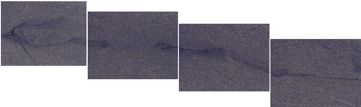
Figure 28 Micrograph of weld area of the sticking sample at 50x magnification
