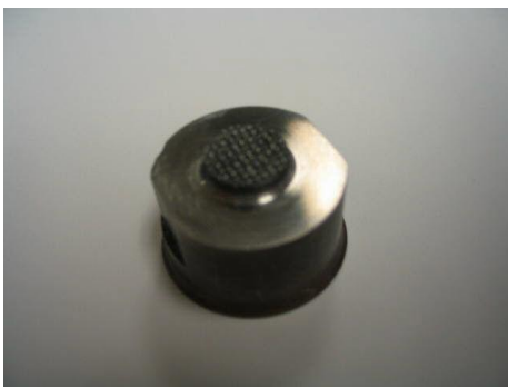
Figure 16 Picture of the anvil knurl pattern (Anvil tip)
