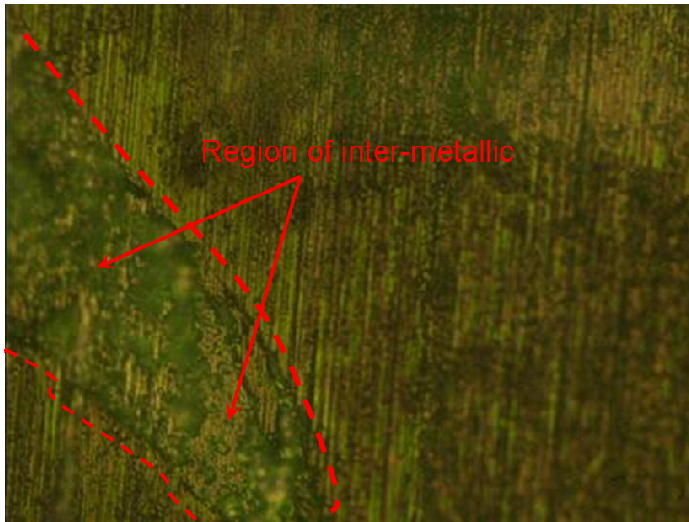
Figure 48 Optical micrographic picture of the inter-metallic layer between the Cu phase and the Al alloy, underneath the horn at 100X
