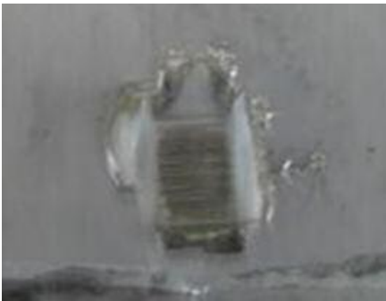
Figure 52 Photograph of part marking without Zn buffer sheets
