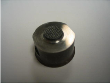
Figure 58 Picture of the anvil tip and knurl pattern
