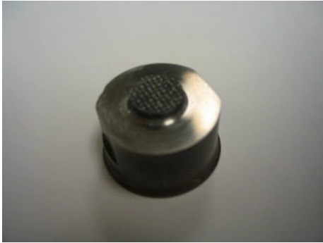
Figure 33 Picture of the anvil knurl pattern (Tip)
