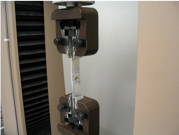
Figure 59 Picture of the testing weld strength
