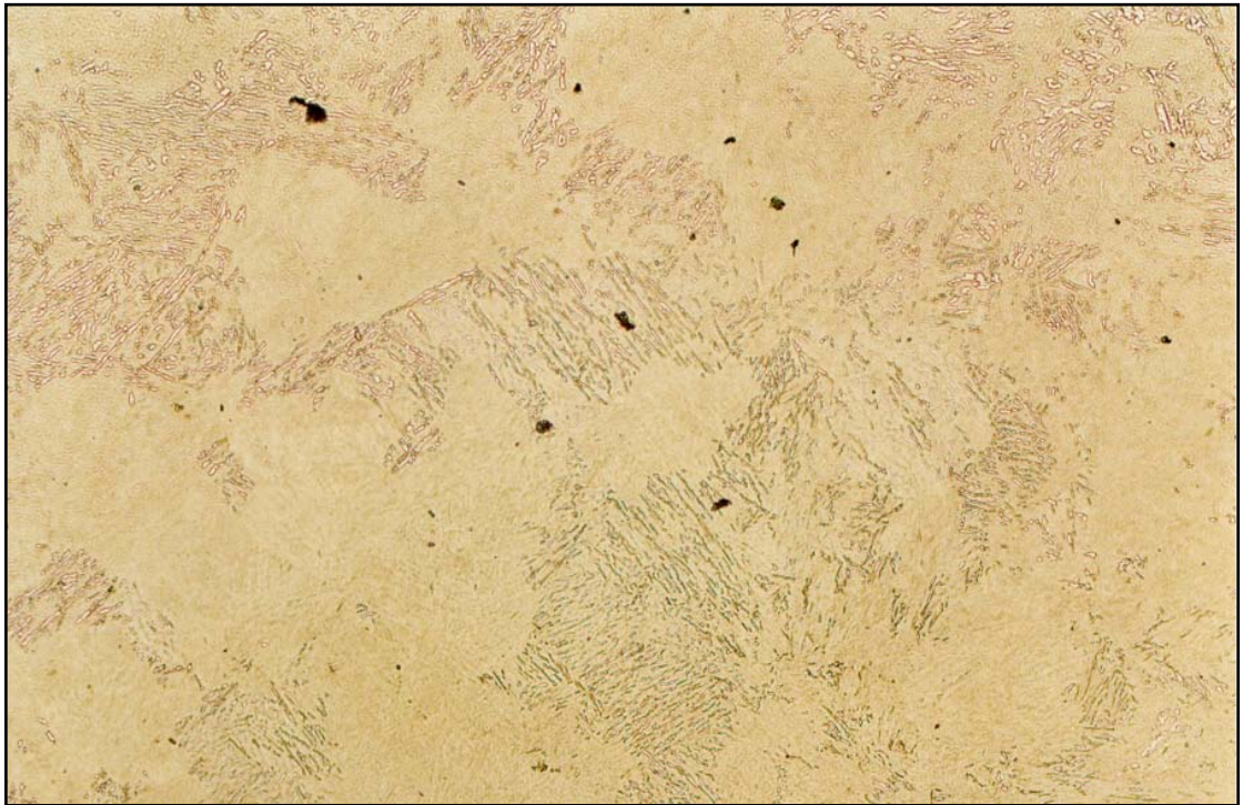
Fig. 5.1: Microstructure of Heat Treated 4340 Steel at 230X
