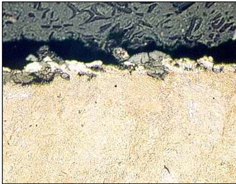
Fig. 6.13: Shot Peened Specimen at 230X
